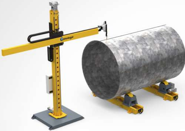
Long Seam welding outside shell
